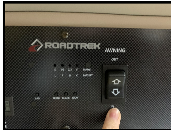
Picture 30.2 The awning power switch
