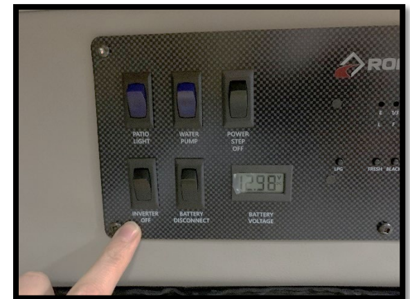
Picture 38.2 Inverter Switch
